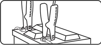
1. Insert the jumper cable into the jump starter and connect the clamps to the car battery.
